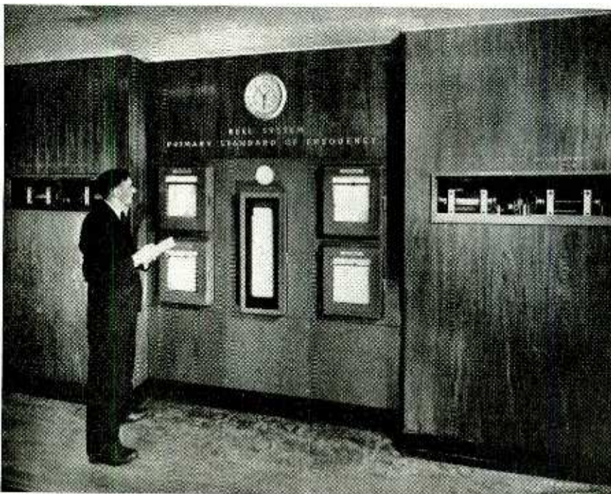
600-tube frequency standard will vary less than one second in next thirty years.
