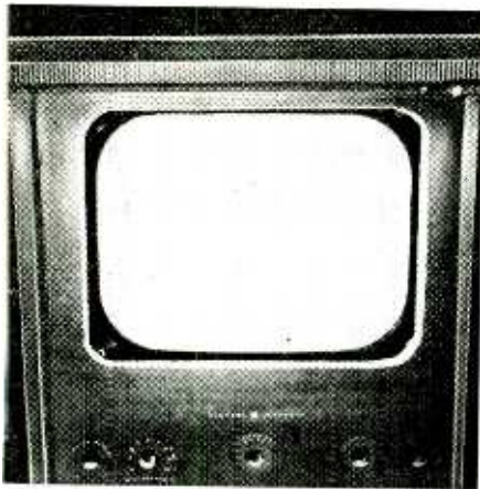
Fig. 3—Cut-out before installing mask.
